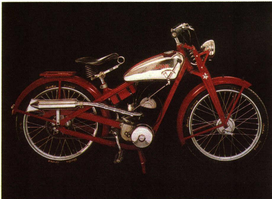
JAWA 100 ROBOT ● Two stroke air-cooled single cylinder with inverted scavenging ● Displacement 98.8 cc (bore and stroke 47×57 mm) ● Engine power 1.9 kW at 3750 r.p.m. ● Compression ratio 5.7 to 1 ● Three-speed gearbox with hand control in unit with engine ● Freewheel permitting rear wheel drive by engine or pedals ● Closed duplex frame made with steel sections ● Rigid rear wheel suspension ● Parallelogram front fork with coil spring suspension ● Weight 49 kg ● Maximum speed 65 km p.h. ● Average fuel consumption 2 litres per 100 km
