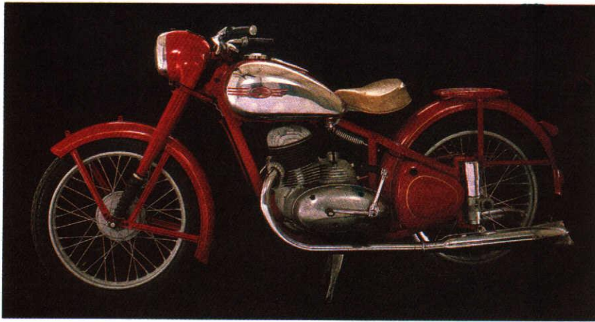
JAWA 250 — Springer ● Two stroke air-cooled single cylinder ● Displacement 248.5 cc (bore and stroke 65×75 mm) ● Engine power 6.6 kW at 4000 r.p.m. ● Four-speed gearbox with foot control in unit with engine ● Multiple clutch in oil bath automatically disengaged by gearchange pedal movement ● Simple closed frame bifurcating at the rear, made with square steel sections ● Rear wheel vertical slider type suspension ● Telescopic front fork ● Weight 115 kg ● Maximum speed 100 km p.h. ● Average fuel consumption 3 litres per 100 km
