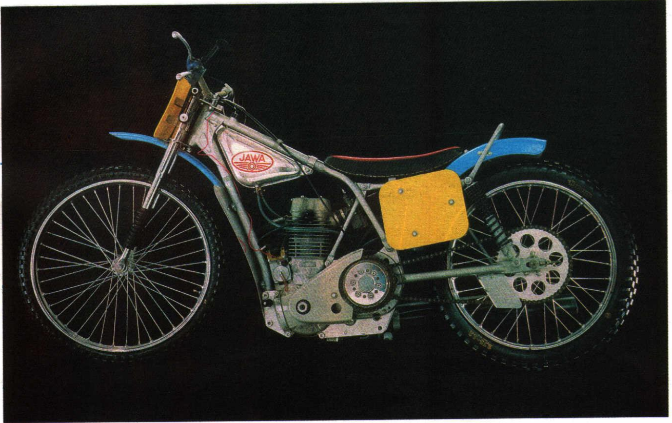
JAWA 500, Model 896 ● Four stroke air-cooled OHC single cylinder ● Displacement 496 cc (bore and stroke 85×87 mm) ● Engine power 48 kW at 8,600 r.p.m. ● Compression ratio 14 to 1 ● Four-valve cylinder head ● Total loss lubrication by double pump ● Two-speed gearbox ● Multiplate dry clutch ● Simple frame welded of steel tubes ● Pivoted rear fork with two oil damped suspension units ● Telescopic front fork ● Weight 93 kg ● Maximum speed and fuel consumption not indicated
