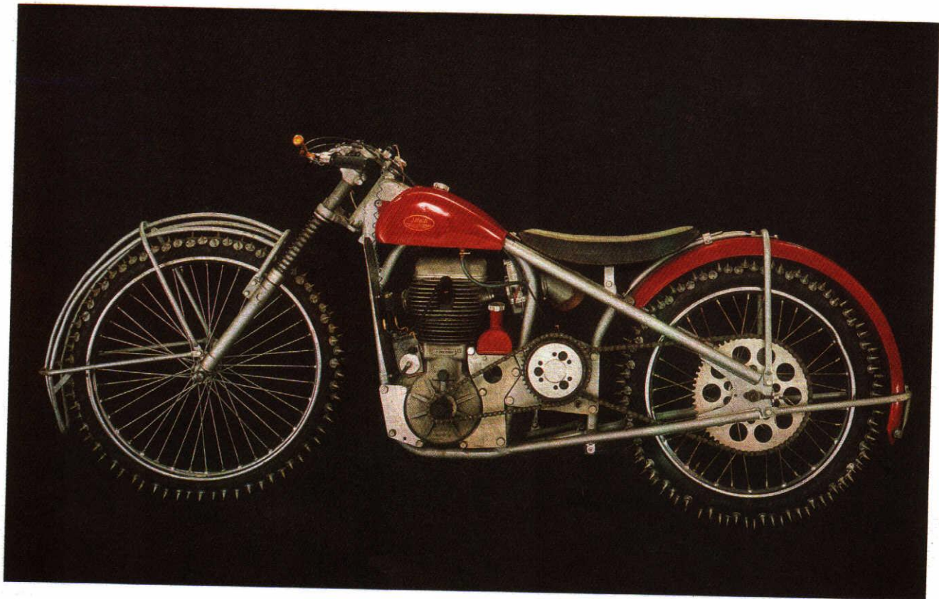
JAWA 500, Model 891 ● Four stroke air-cooled OHV single cylinder ● Displacement 497 cc (bore and stroke 88×81.7 mm) ● Engine power 36.8 kW at 7250 r.p.m. ● Compression ratio 14 to 1 ● Two-valve cylinder head ● Total loss lubrication by double pump ● Oil tank situated aft of the engine ● Two-speed gearbox with foot control ● Simple closed frame welded of steel tubes ● Rear wheel without spring suspension ● Telescopic front fork ● Weight 128 kg ● Maximum speed and fuel consumption not indicated
