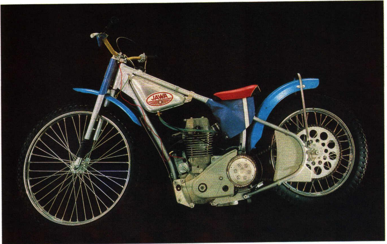
JAWA 500, Model 897 ● Four stroke air-cooled OHC simple cylinder ● Displacement 496 cc (bore and stroke 85×87) ● Engine power 44 kW at 8,600 r.p.m. ● Compression ratio 13 to 1 ● Four-valve cylinder head ● Total loss lubrication by double pump ● Multiplate dry clutch ● Simple frame made with steel tube; central and rear part bolted ● Rear wheel without spring suspension ● Telescopic front fork ● Weight 83 kg ● Maximum speed and fuel consumption not indicated
