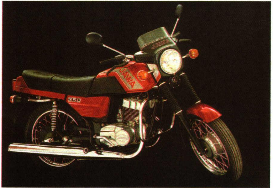
JAWA 350, Model 638 ● Two stroke air-cooled twin cylinder ● Displacement 343.5 cc (bore and stroke 58×65 mm) ● Engine power 19 kW at 5250 r.p.m. ● Compression ratio 10.2 to 1 ● Four-speed gearbox with shifting gears ● Multiplate clutch in oil bath ● Duplex cradle type frame made with circular section steel tubes ● Pivoted rear fork with two oil damped suspension units ● Telescopic front fork ● Weight 156 kg ● Maximum speed 125 km p.h. ● Average fuel consumption 4.5 litres per 100 km
