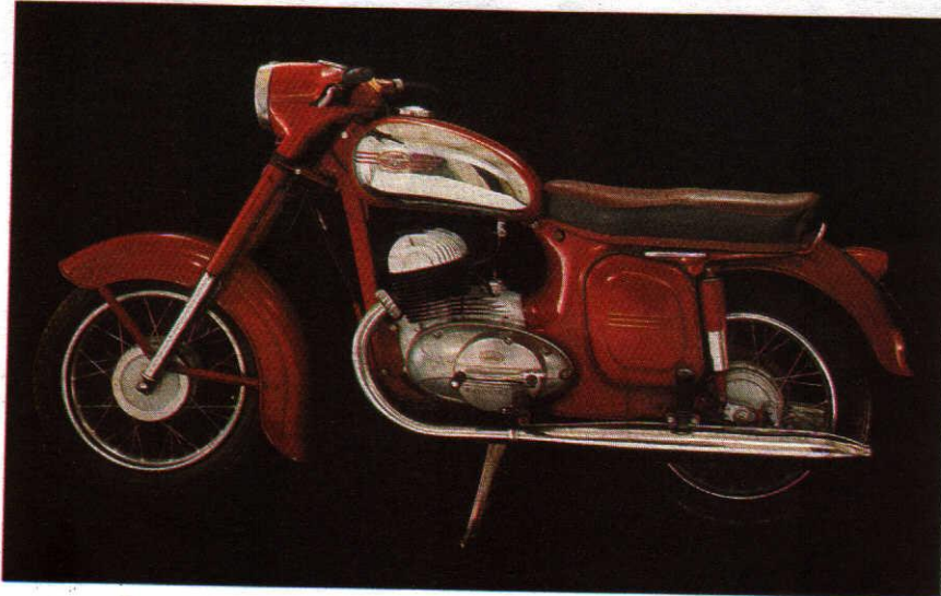
JAWA 350 Automatic, Model 360 ● Two stroke air-cooled twin cylinder ● Displacement 344 cc (bore and stroke 58×65 mm) ● Engine power 12.5 kW at 5000 r.p.m. ● Compression ratio 8.2 to 1 ● Four-speed gearbox ● Automatic centrifugal clutch ● Simple closed frame welded of square steel sections ● Pivoted rear fork with two oil damped suspension units ● Telescopic front fork ● Weight 150 kg ● Average fuel consumption 3.5 litres per 100 km
