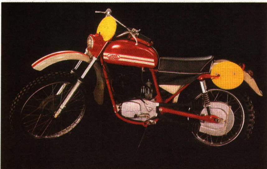
JAWA 250, Model 652 ● Two stroke air-cooled single cylinder ● Displacement 246 cc (bore and stroke 70×64 mm) ● Engine power 20.6 kW at 7000 r.p.m. ● Six-speed gearbox ● Multiplate dry clutch ● Crankshaft assembly and gearbox fitted in the crankcase from the side ● Duplex cradle type frame welded of chrome-molybdenum circular section tubes ● Pivoted rear fork with two oil damped suspension units and progressive coil springs ● Telescopic front fork ● Weight 118 kg ● Maximum speed 135 km p.h. ● Fuel consumption not indicated
