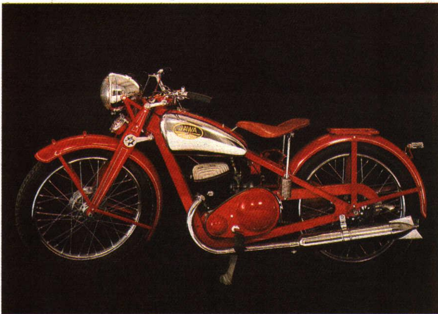
JAWA 175 Special ● Two stroke air-cooled single cylinder with inverted scavenging ● Displacement 173 cc (bore and stroke 58×65 mm) ● Engine power 4.5 kW at 3750 r.p.m. ● Compression ratio 6.2 to 1 ● Separate three-speed gearbox with foot control ● Dry multi-plate clutch ● Closed duplex frame made with steel stamped sections ● Rigid rear wheel suspension ● Parallelogram front fork with coil spring suspension ● Weight 97 kg. Maximum speed 90 km p.h. ● Average fuel consumption 3 to 3.5 litres per 100 km
