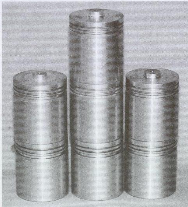
Piston Blanks with Lathe Operations Completed
