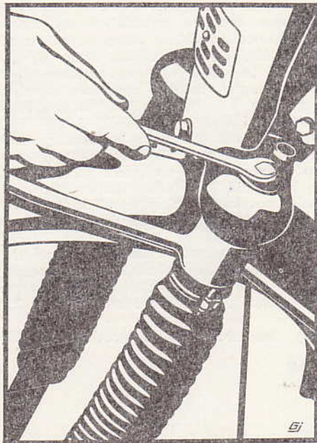
14 - Removal of front telescopic fork
