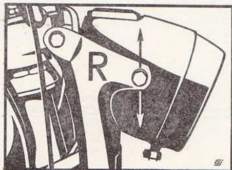
39 – Vertical adjustment of headlights
