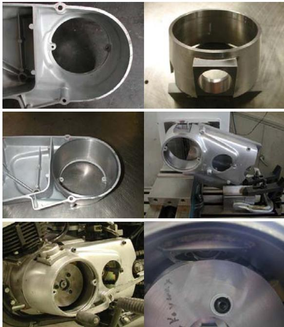
Figure 3: Upper Left - Stock cast aluminum case Upper Right - Machined ring with welded boss Middle Left - Ring epoxied into cast aluminum case Middle Right - Finish machining of case Lower Left - Modified case mounted to engine Lower Right - Air compressor follower riding on cam
