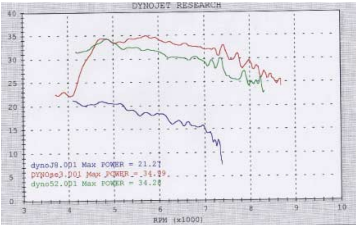
Comparison of power for the stock pipe, ideal prototype and final pipe
